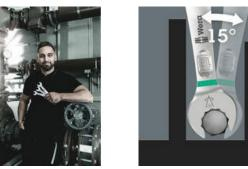
The Joker 6003 ring spanner with its special mouth geometry mouth side pivoted by 7.5° and the double hexagon profile doubles the placement possibilities when repeatedly turning the wrench 180° around the longitudinal axis. Bolts and screw heads can be "accessed" every 15°. The Joker 6003 will automatically find the respective placement point after every turn.
